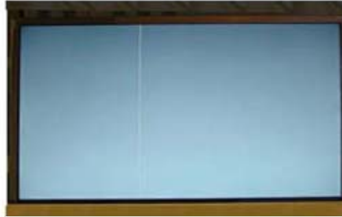
Vertical Line Source TAB IC Defect
