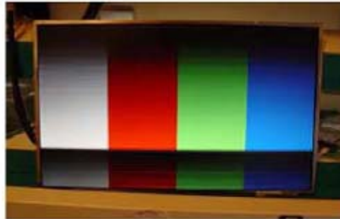
Horizontal Block Gate TAB IC Defect
