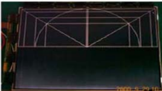
Horizontal Block Gate TAB IC Defect
