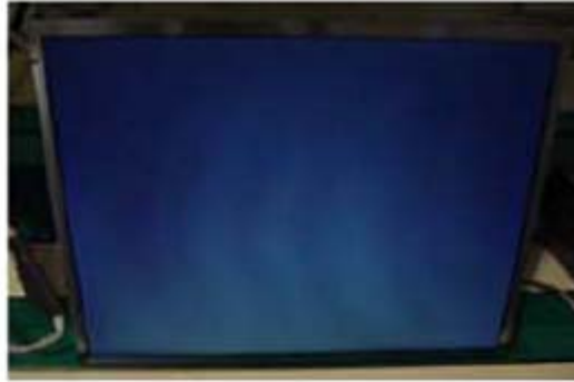
Panel Mura, Light leakage
