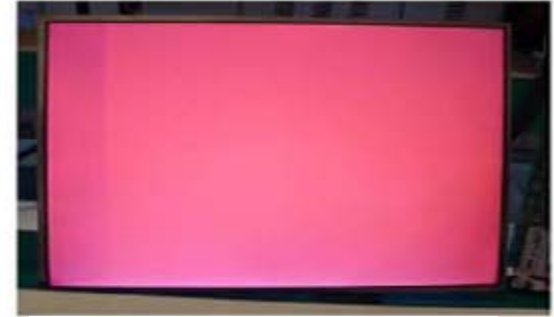
Vertical Block Source TAB IC Defect
