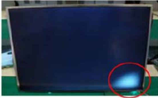
Panel Mura, Light leakage
