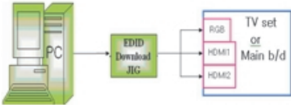
(Fig. 2) Connection Diagram of DDC download
