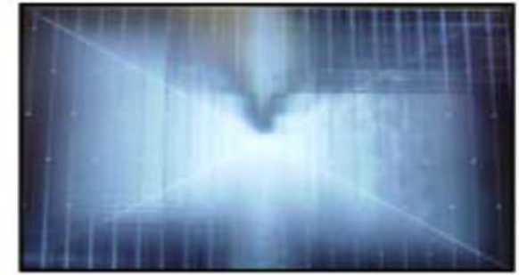
Solder defect, Short/Crack
