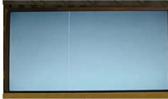
Vertical Line Source TAB IC Defect
