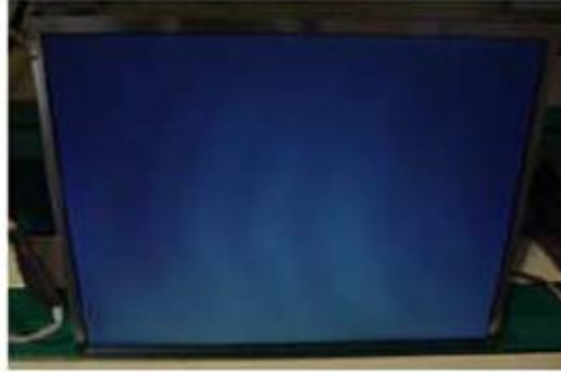
Panel Mura, Light leakage
