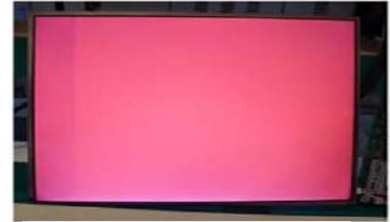
Vertical Block Source TAB IC Defect
