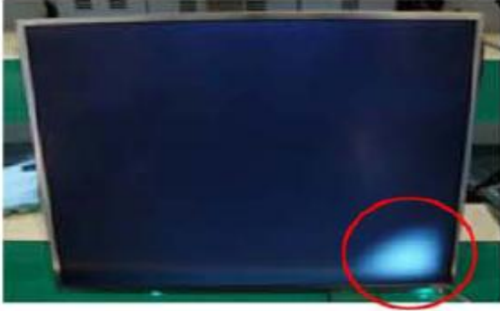
Panel Mura, Light leakage
