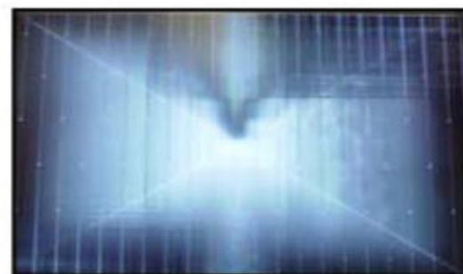
Solder defect, Short/Crack
