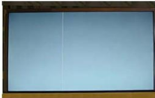
Vertical Line Source TAB IC Defect
