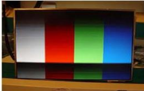
Horizontal Block Gate TAB IC Defect
