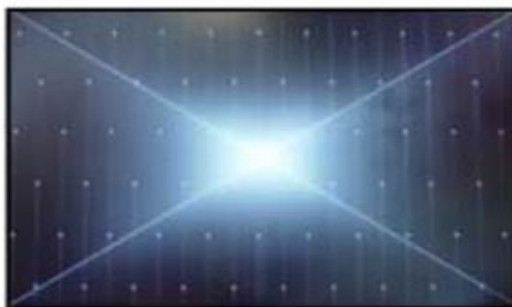
Solder defect, Short/Crack
