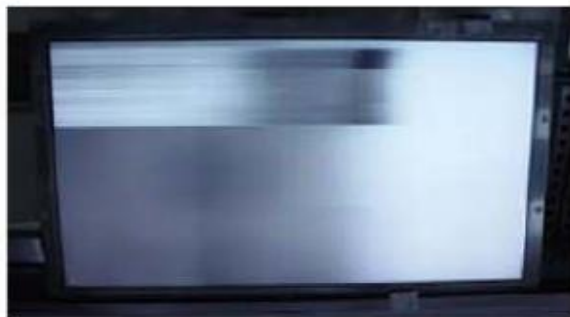
Horizontal Block Gate TAB IC Defect
