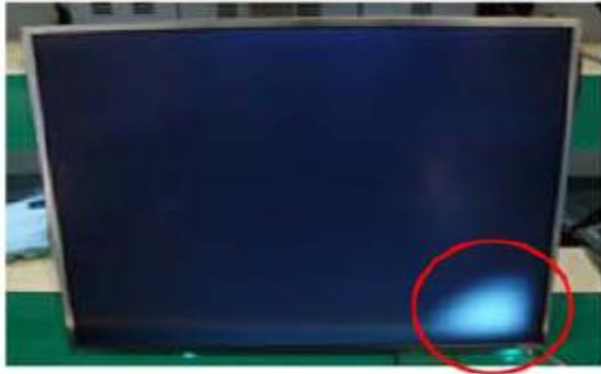
Panel Mura, Light leakage
