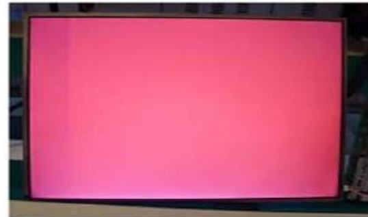
Vertical Block Source TAB IC Defect
