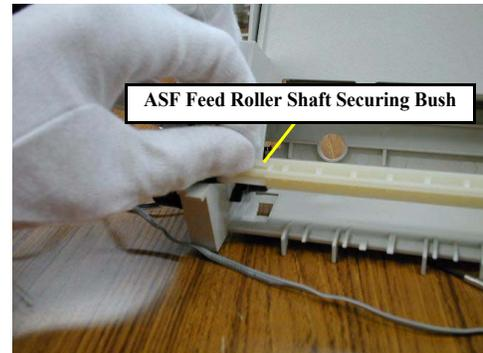
Figure 7-26. Removal of ASF Feed Roller Securing Bush
