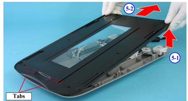
Figure 4-28. Removing TPU Lower Housing (2)
