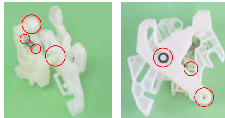
Figure 4-89. Reassembling the Right CD-R Release Lever Sub Assy
