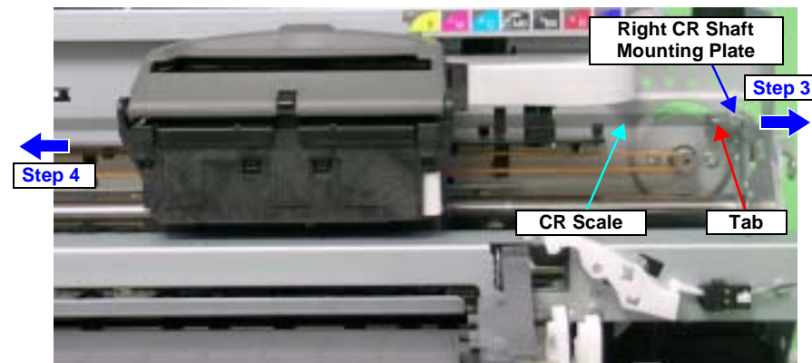
Figure 4-38. Drawing Out the CR Scale
