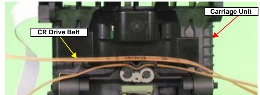
Figure 4-69. Removing the CR Drive Belt
