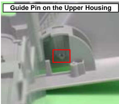
Figure 4-10. Removing the Printer Cover
