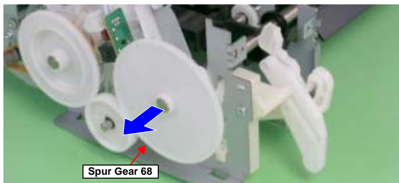
Figure 4-91. Removing the Spur Gear 68
