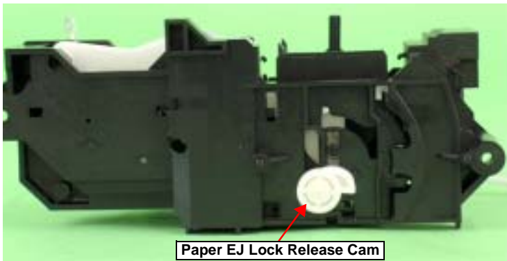
Figure 4-102. Installing the Paper EJ Lock Release Cam
