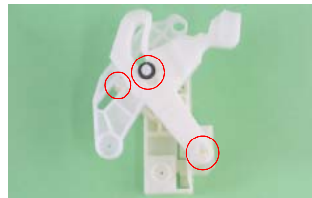
Figure 4-93. Reinstalling the Left CD-R Release Lever Sub Assy (1)
