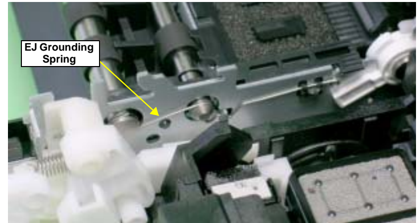
Figure 4-114. Removing the EJ Grounding Spring
