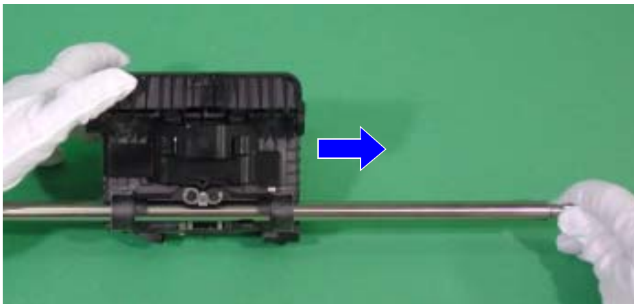
Figure 6-18. Lubricating the Carriage Shaft (5)
