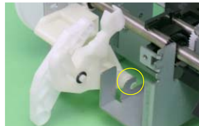
Figure 4-94. Removing the Left CD-R Release Lever Sub Assy (2)
