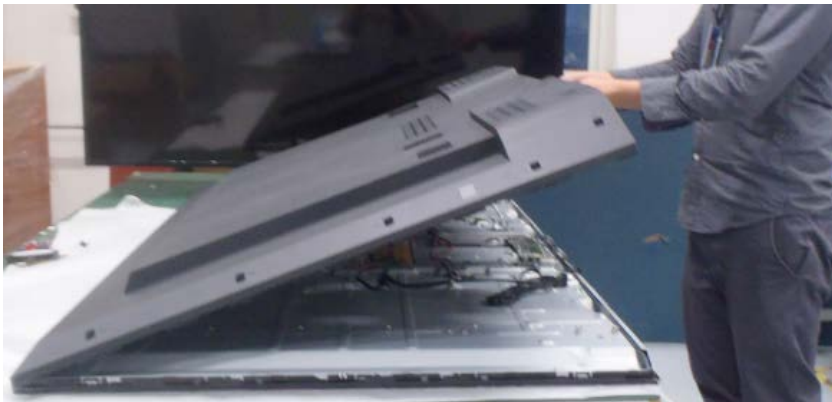
Lift up the rear cover from the bottom
