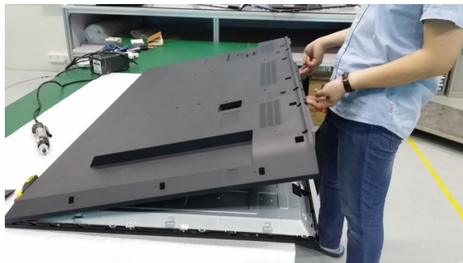
Lift up the rear cover from the bottom
