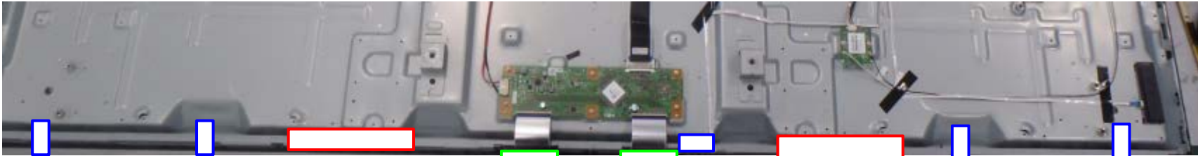
Peel off bottom Aluminum tape.
