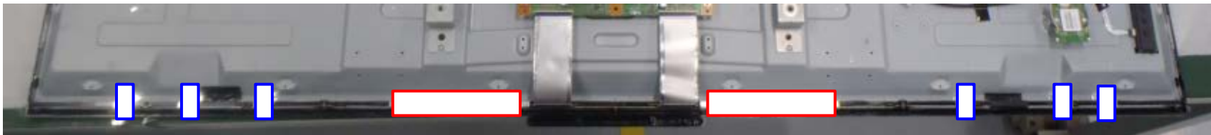
Peel off bottom Aluminum tape.
