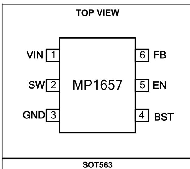
**MPS** MP1657 – SYNCHRONOUS, STEP-DOWN CONVERTER WITH INTERNAL MOSFETS
