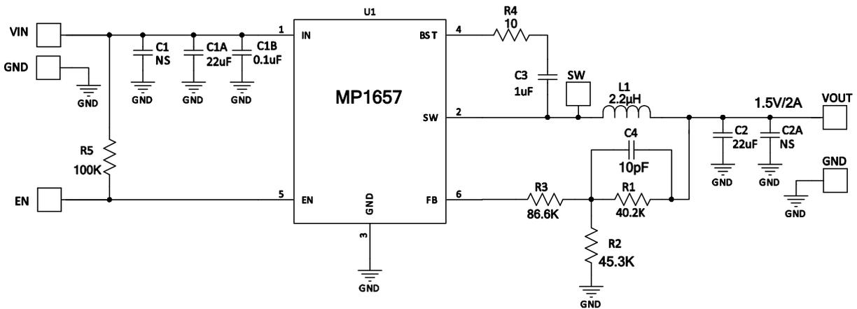
Figure 10: 12VIN, 1.5V/2A Output
