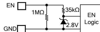
**Figure 2: Zener Diode between EN and GND**
