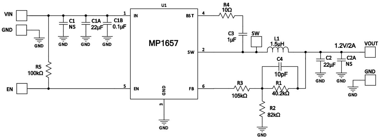
Figure 11: 12VIN, 1.2V/2A Output
