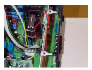
The compensation cable, which is soldered in at pin 7 of the diode split transformer, has to be passed trough the hole at pin 1 to the ferrit tube. The compensation cable has to be fixed with two cable ties in the middle of the ferrit tube, runed between the cooling shield and the screening of the signal P.C. board and soldered in at the frame of tuner.
