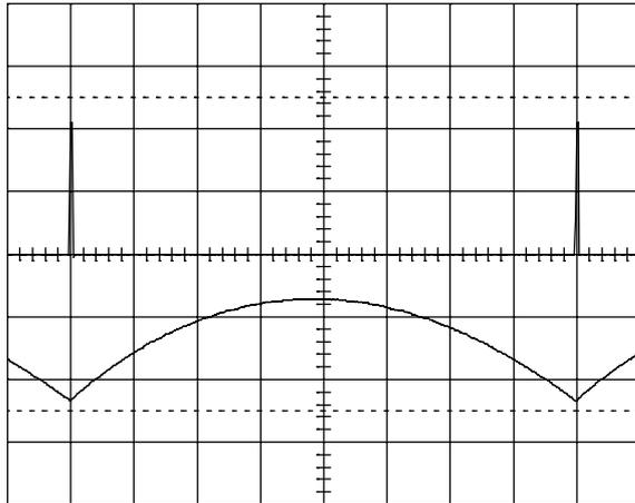
Top trace: Vblank at connector 1 pin 5.
