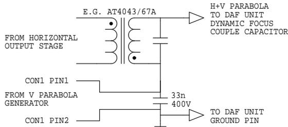
To prevent semiconductor destruction during a flash, it is of great importance that the 33nF capacitor is placed close to the horizontal parabola generator, and connected directly to the DAF unit. The two traces (wires) of the vertical output parabola with the ground (connector 1 pins 1 and 2) must be kept close together and connected directly across the 33nF capacitor.
