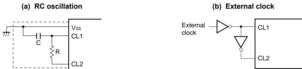
Figure 5-9. External Circuit of External RC Oscillator
