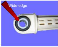
When inserting the damper into its seat (in the lower section of the cabinet or the tub), ensure that the ferrule is correctly positioned. The pin should be inserted from the side on which the lip of the ferrule is wider. The ferrule is available as a spare part (part no. 344 91 25-30/59.
