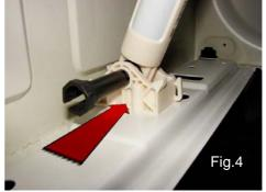
If difficulty is encountered when inserting the pin (fig. 4), apply a small quantity of grease (Cod. 5026 24 16-00/6)
