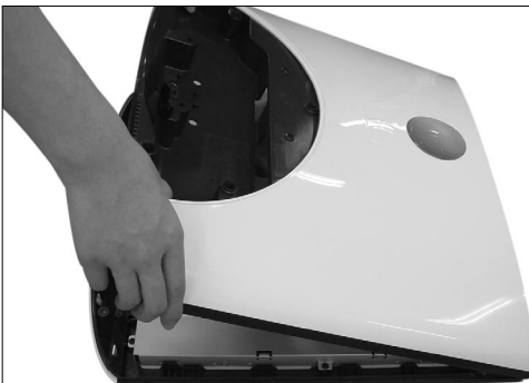
Disassemble back cover.
