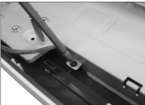
Remove the 7 screws from each side of metal frame.
