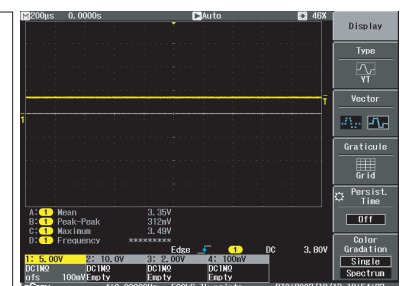
⑥ CVBS Waveform IC2 Pin(9,90,95,100,101)
