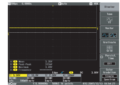
4 CVBS Waveform ZIC1 Pin(54,56,59,62)
