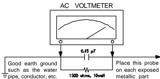
AC Leakage Current Check
