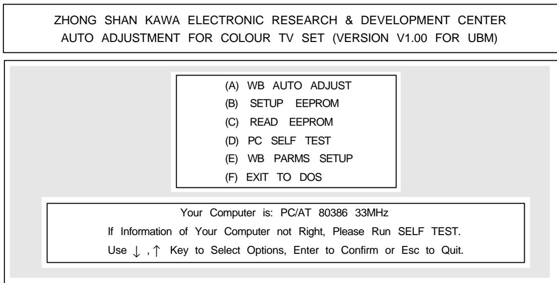
This is the main menu for adjustment and the different data can be changed and viewed. It consists of following functions.
