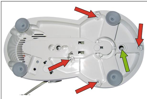
3. Remove the 2 last screws (marked with the red arrows). After this you can remove the housing.
