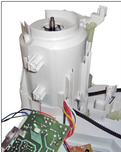
After removing the Airtunnel, you can exchange the motor, the belt or the belt tension.
