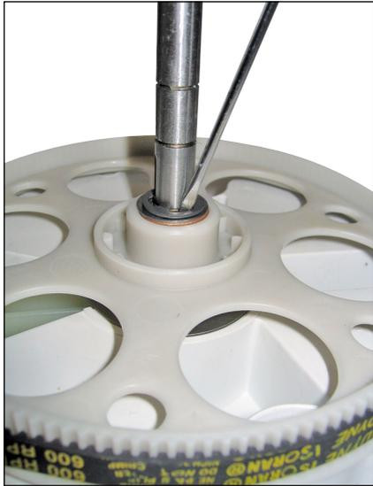
Remove the Belt tension, by lifting it a little bit (green arrow) and pulling it in direction of the red arrow.
