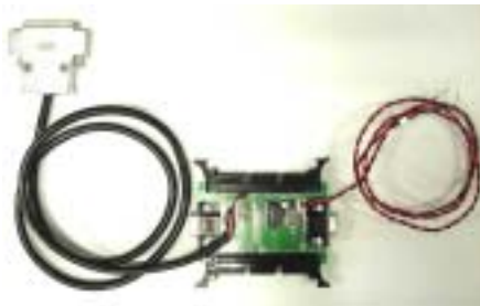
DDC Communication I/F BOARD (Part No.: 599910541)
