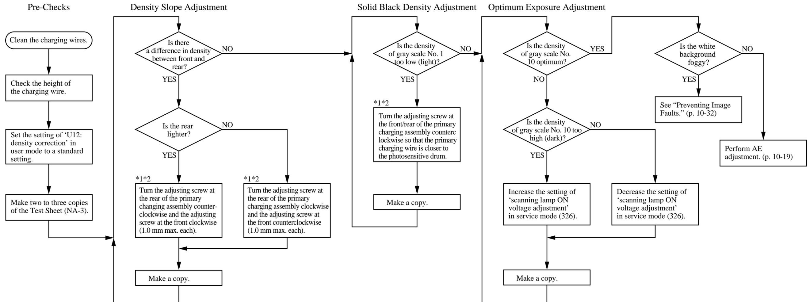
1: If there still is a difference after turning the adjusting screw 1.0 mm each\*, check the charging assembly, scanning lamp, and scanner for dirt.
