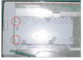
Separate the lamp shield from rear shield. Please pull off the latch first.
