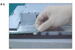
Remove the control button from cabinet, Then disassemble the connector.
