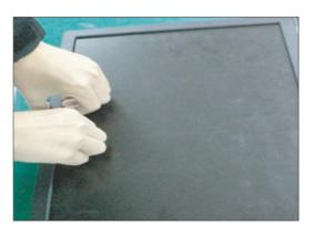
Pull the cabinet upwards, Then separate all latches on each side.
