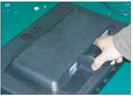
Disassemble the back cover.
