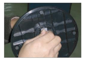
Turn around the base lock to open the lock between base cover and stand body...
