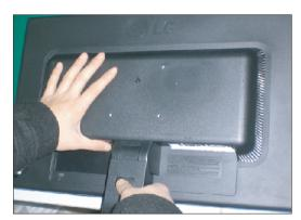
Pull the cabinet upwards, Then push the button "push" to separate the hinge body and stand body.
