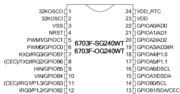
Figure 8-2 Internal block diagram and pin configuration
