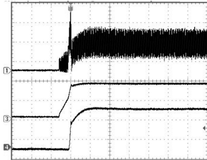
Startup Plot ( V_{IN} = 3.6V , I_{LED} = 19mA , L = 22\mu H , Ramp Rate = 8\mu s/step )
