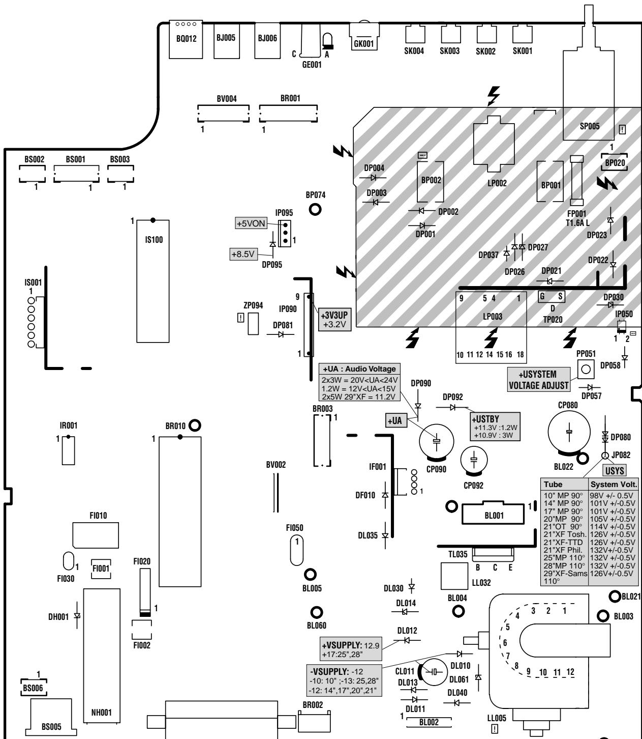
Part of board connected to mains supply.
