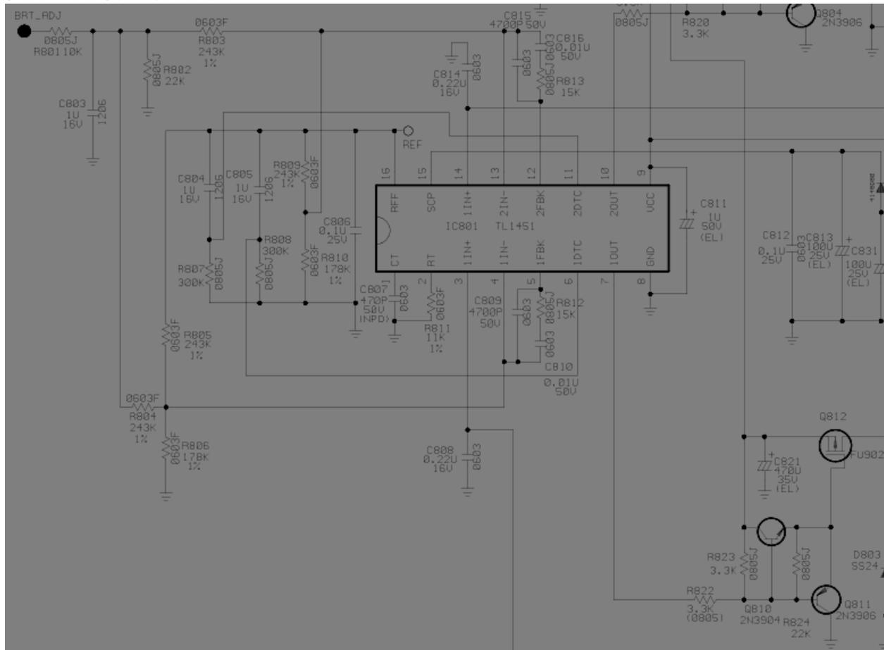
TL1451 is a dual PWM controller. C807 and R811 decide the working frequency. BLT\_ADJ signal is from control board, control pulse width then decide how much energy delivery to CCFL also decide CCFL brightness. Q810 and Q811 be the buffer to rise the drive capability and the totem poles circuit can improve a capable of driving for Q812. C813 decide the striking time delay.
