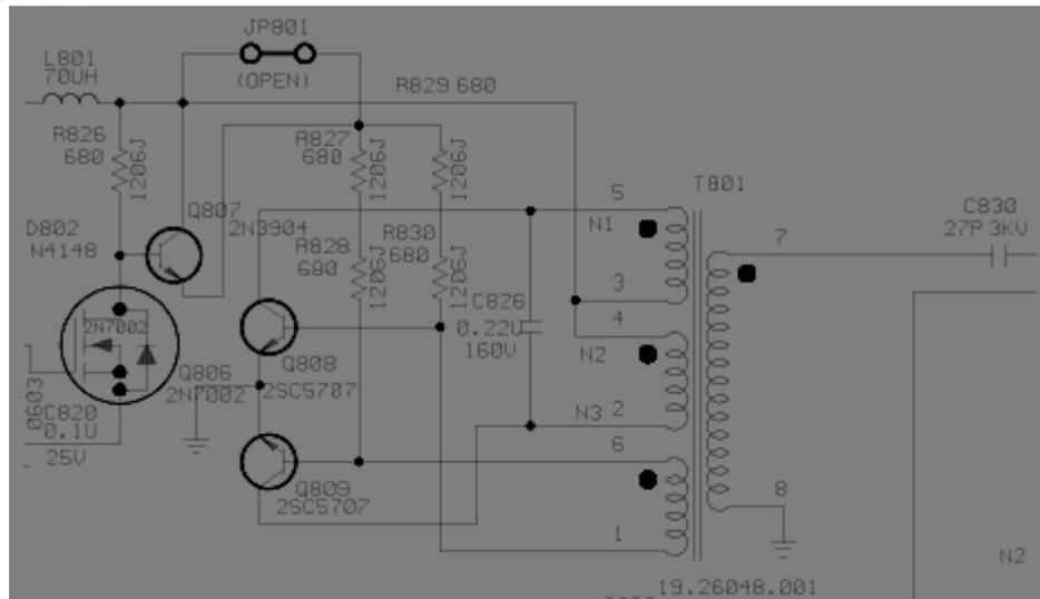
Royer circuit uses the characteristic of transformer saturation to oscillate. When the DC power inject, Q808 or Q809 will turns on, and the current  $I_c$  increases. After a period, the transistor will leave the saturation status and  $V_{ce}$  increase. The result causes the voltage of primary coil get lower. Finally the transistor turn off, and another transistor turn on. These statuses are repeated and the pin7 and pin8 of T801 will get a sine wave to turn on CCFL.
