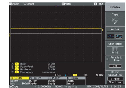
4 CVBS Waveform ZIC1 Pin(54,56,59,62)
