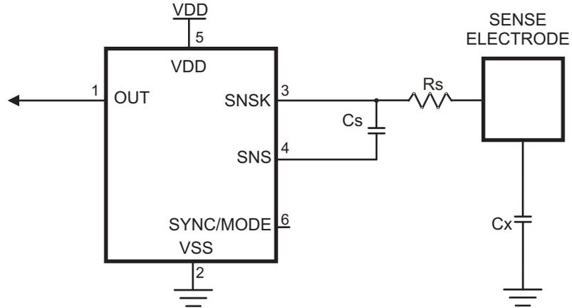
Note: A bypass capacitor should be tightly wired between Vdd and Vss and kept close to pin 5.
