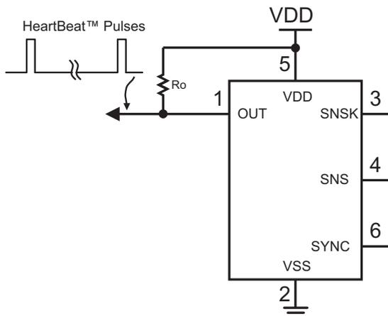
If the sensor is wired to a microcontroller as shown in [Figure 3-7 on page 11](#), the microcontroller can reconfigure the load resistor to either Vss or Vdd depending on the output state of the QT1011, so that the pulses are evident in either state.
